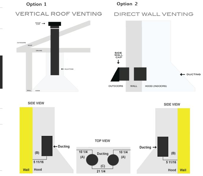
A - 10 1/4'' from the side edge of the hood to the center of the duct
