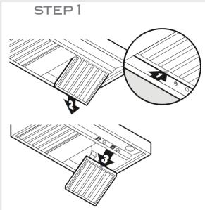
Slide filter forward off of rear lip. Lower filter rear, then slide filter front out. Repeat this step for all filters on the front and back of the hood.
