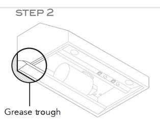
When cleaning filters, always remove the grease channels and clean with hot soapy water. Both the filters and the channels are dishwasher safe. Dry throughly before re-installing.
