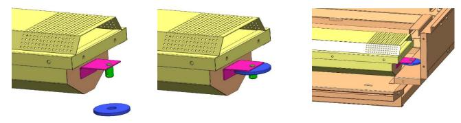
5. With either of the above configurations, replace the cotter pin to hold the burner firmly in place.
