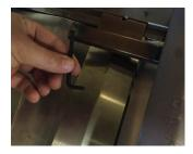
4. Install the infrared burner into the grill in the same way that the conventional burner installed with the male post on the rear of the burner resting in the opening in the grill chassis and the cylindrical venture tube installing around the valve stem in the front. Note: IT IS CRITICAL THAT THE FRONT END OF THE INFRARED BURNER IS INSTALLED APPROPRIATELY ONTO THE GAS VALVE TO ENSURE THE GAS FLOWS SAFELY INTO THE BURNER.
